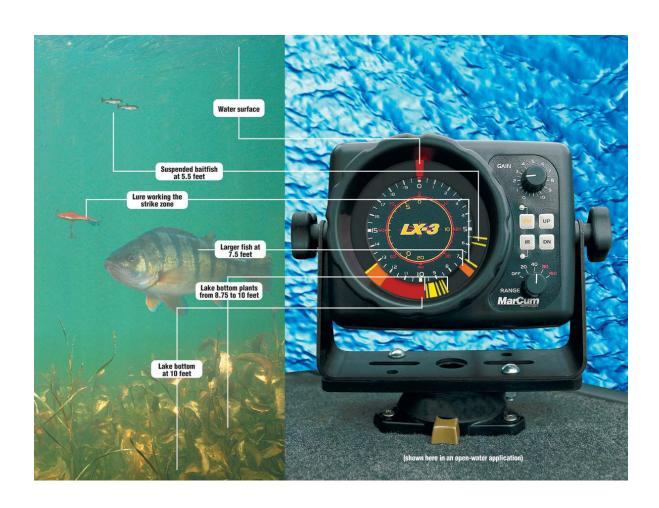
To check the location, press either the UP key or the DN key to activate the visual blinking lights to reacquaint yourself with the location. The blinking yellow lights only assist you in setting the location and act as a visual reference.
